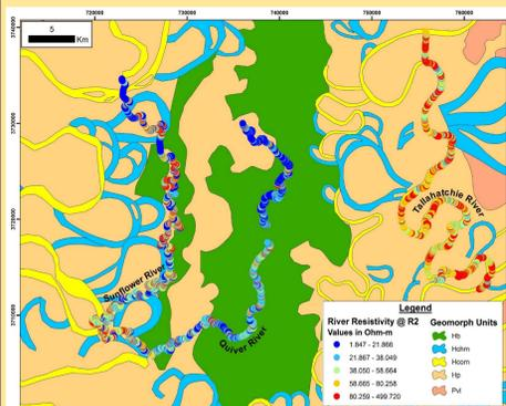
Figure 3: Qualitative estimate of streambed hydraulic conductivity from waterborne resistivity values for surveyed rivers overlain on geomorphology, map citation 2.
