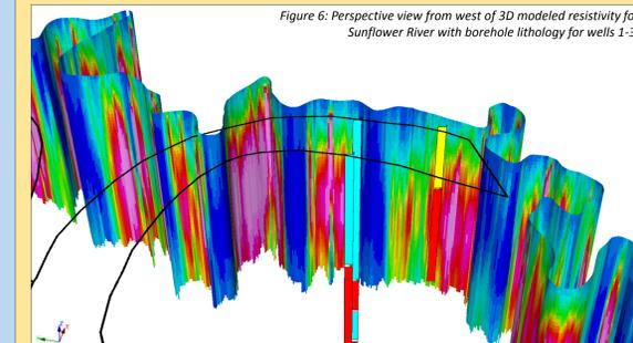
Figure 6: Perspective view from west of 3D modeled resistivity for Sunflower River with borehole lithology for wells 1-3.
