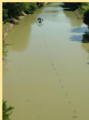
Figure 2: Waterborne-resistivity survey in-progress on Quiver River, Photo by author
